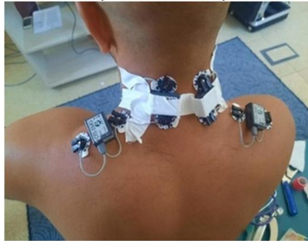
Figure 6. Sensor placement for EMG recordings.
