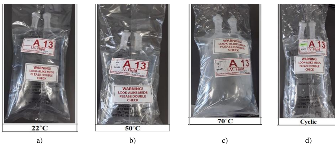
Figure 2. Swelling of polyolefin (PLUMAT) normal saline bags under different temperature conditions: (a) 22 °C, (b) 50 °C, (c) 70 °C, and (d) cyclic temperature exposure.
