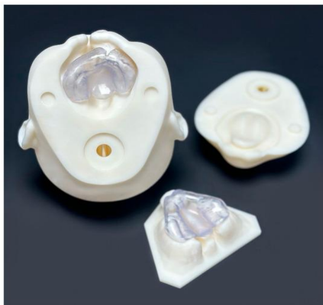
Figure 2. Top left: phantom head with unilateral cleft and inserted maxillary plate; top right: detached lower jaw section; bottom center: 3D-printed model of bilateral CLP fitted with the maxillary plate
