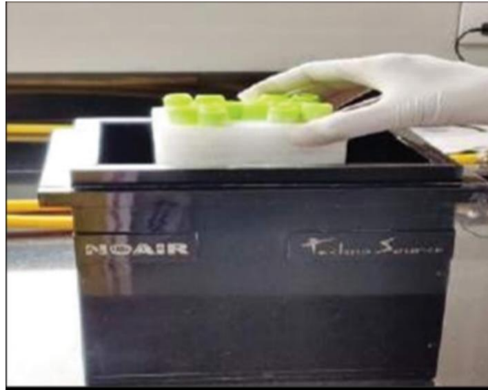
Figure 4. Vials containing Porphyromonas gingivalis contaminated implants placed in an anaerobic jar
