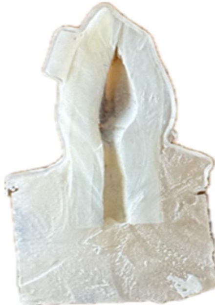
Figure 2. Cross-sectioned tooth sample
