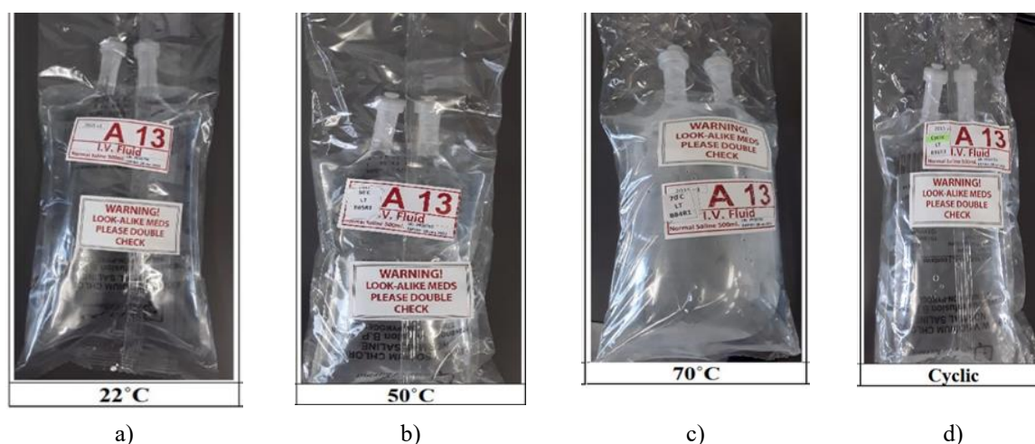
Figure 2. Swelling of polyolefin (PLÜMAT) normal saline bags under different temperature conditions: (a) 22 °C, (b) 50 °C, (c) 70 °C, and (d) cyclic temperature exposure.
