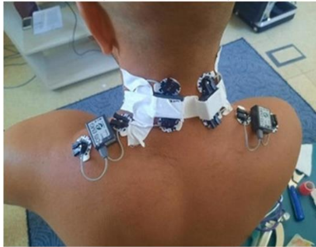
Figure 6. Sensor placement for EMG recordings.
