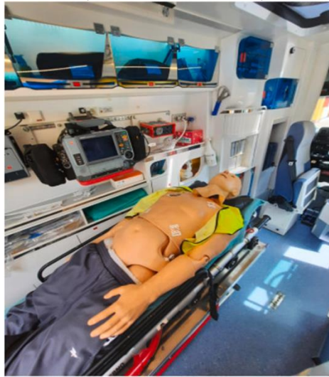
Figure 1. Test setup – interior of a fully equipped ambulance with a stretcher-mounted medical simulator.
