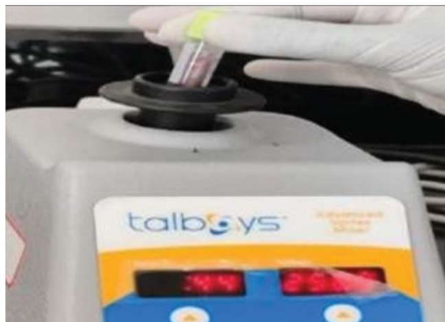
Figure 6. Agitation of disinfected implants in ten milliliters of thioglycolate broth for 60 seconds
