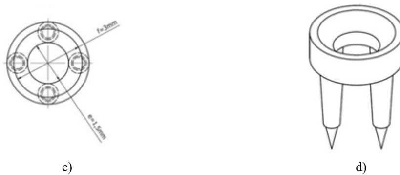
Figure 3. A technical drawing of the SD—(a) front view (elevation view); (b) sectional view (cut along A-A); (c) top view (plan view); (d) isometric view. Legend—a: ring height of 6 mm; b: ring diameter of 4 mm; c: maximum insertion size into the bone of 1 mm; d: leg height of 4 mm; e: internal diameter of 1.5 mm; f: external diameter of 3 mm.
